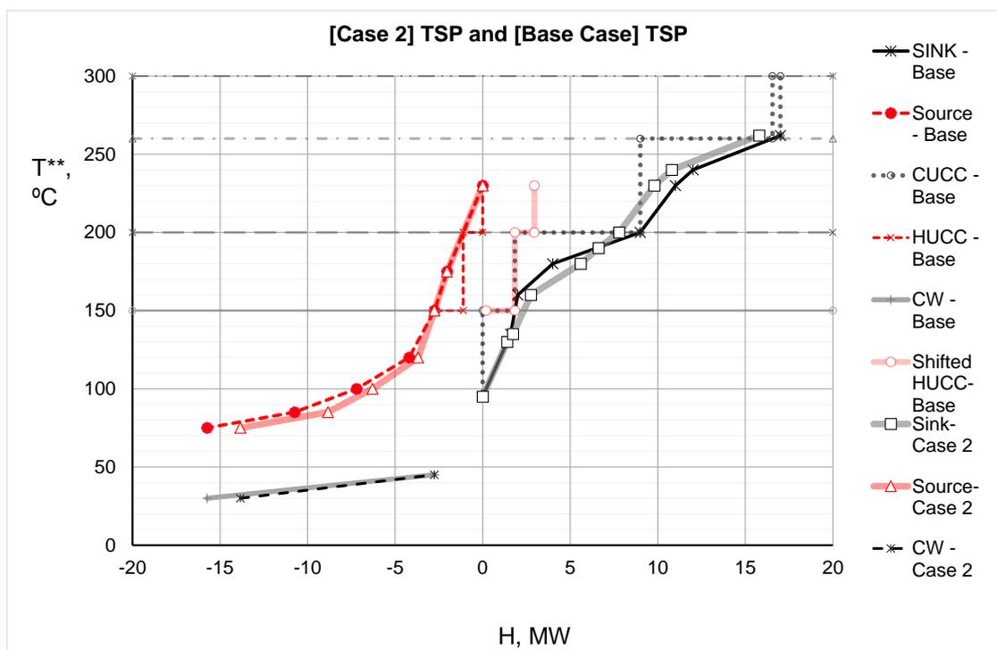
Figure 5: Changed TSP with application of KHSH/KCSC as in Case 2
