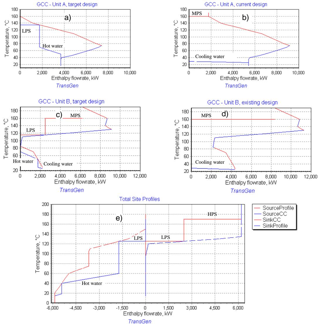
Figure 3: GCCs for target and existing designs for Plant A (a, b), B (c, d), and TS Profiles
