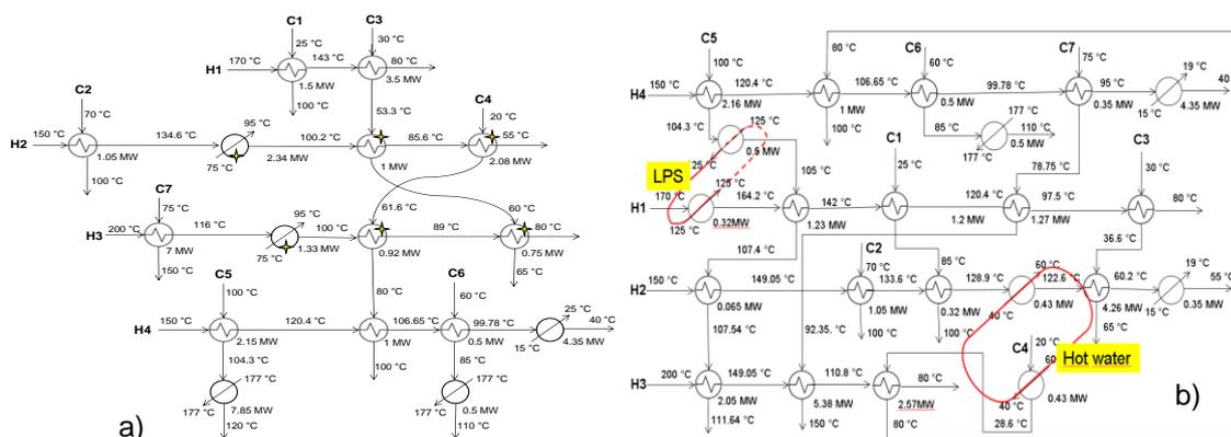
Figure 5: Examples of HEN designs for TS when performing modifications of HEN for: a) direct heat transfer by modifying the existing HEs and b) indirect heat transfer by modifying five existing HEs
