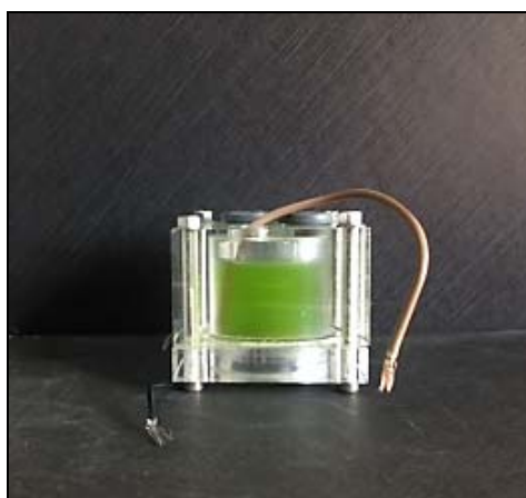
Figure 2: Biophotovoltaic cell experimental setup
