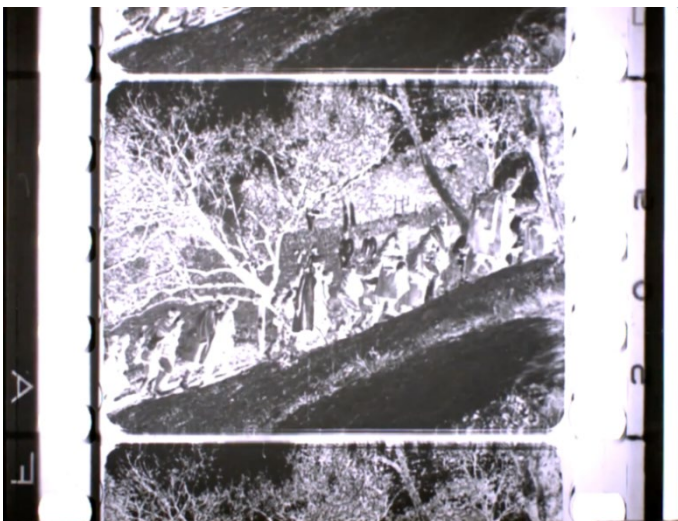
Fig. 2. example of an edge-to-edge taken from reel 1 of witness "RM" (frame 3093); even if it is a negative copy, it is possible to identify the overlapping of the positive perforations; it shows the Producers' Edge Marks "AGFA" on the left and the numbers "509" that are a part of the edge code, on the right.
