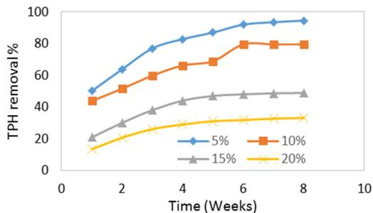
Fig. 4. Effect of activated sludge, NPK fertilizer and coconut shell powder on TPH removal
