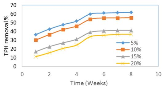
Fig. 2. Effect of activated sludge and coconut shell powder addition on TPH removal
