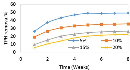
Fig. 1. Effect of coconut shell powder addition on TPH removal
