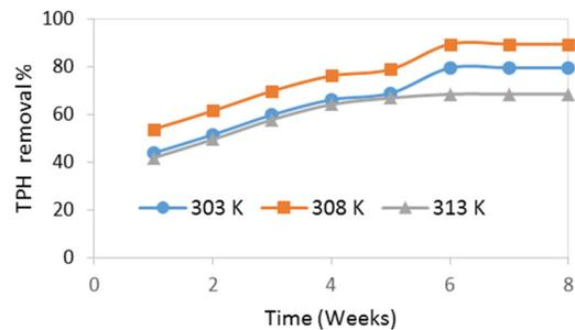
Fig. 5. Effect of operating temperature on TPH removal.
