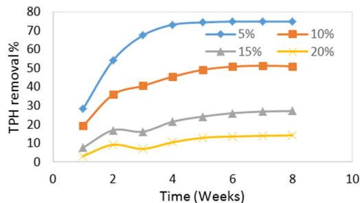
Fig. 3. Effect of NPK fertilizer on TPH removal
