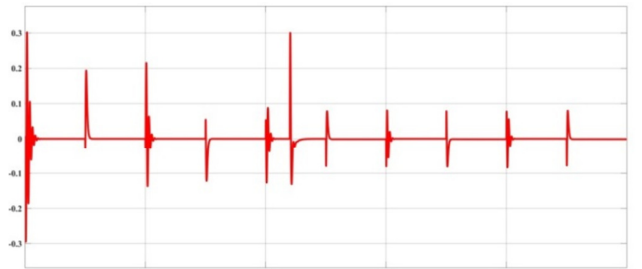
Fig. 10. Error change in LQR assisted adaptive control system for varying load at the 110 th second
