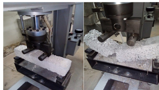
Fig. 2. View of a prism sample before and after testing in UTM
