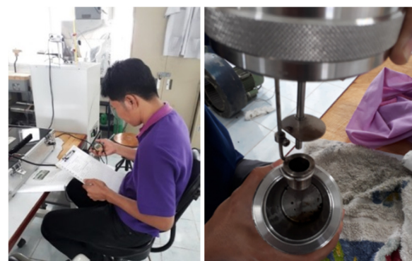
Fig. 5. Bomb calorimeter for heating value measurements.
