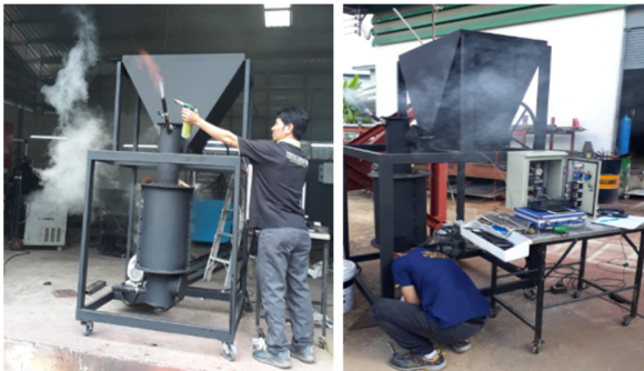
Fig. 6. Gasifier startup and operation.
