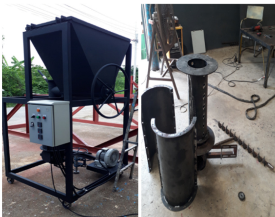
Fig. 3. Updraft Gasifier 80kW prototype and its fabrication.
