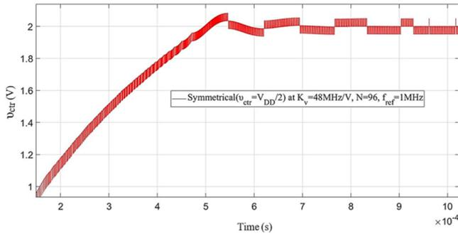
Fig. 1. Symmetrical transient behavior of the VSCP-PLL.
