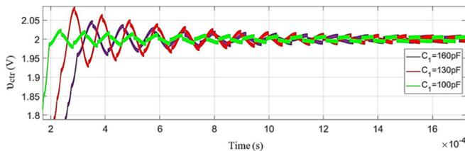
Fig. 5. Transient behavior of VSCP-PLL at different values of  $C_1$  ( $V_{DD}=4V$ ,  $R_0=2M\Omega$ ,  $f_{ref}=1MHz$ ,  $N=96$ ,  $K_v=48MHz/V$ ,  $R_1=10K\Omega$ ,  $C_I=100pF, 130pF$ , and  $160pF$ ).
