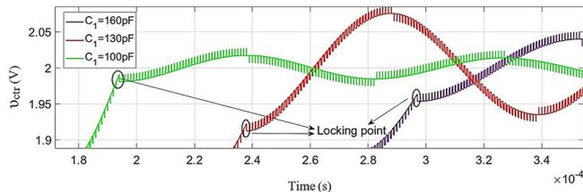
Fig. 6. Impact of varying capacitor  $C_1$  of the LF on the locking time of VSCP-PLL.
