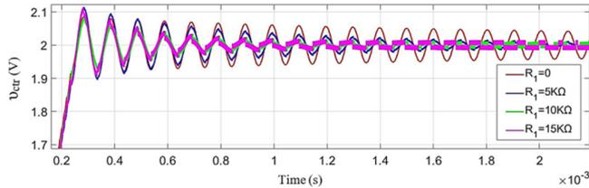
Fig. 4. Transient behavior of VSCP-PLL at different values of  $R_1$  ( $V_{DD}=4V$ ,  $R_0=2M\Omega$ ,  $f_{ref}=1MHz$ ,  $N=96$ ,  $K_v=48MHz/V$ ,  $R_I=10K\Omega$ ,  $R_1=0, 5K\Omega, 10K\Omega$  and  $15K\Omega$ ).
