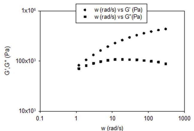
Fig. 1. Frequency sweep test for sPP/S-2 at 200°C.
