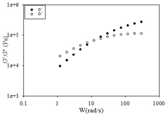
Fig. 2. Frequency sweep test for sPP/S-6 at 200°C.
