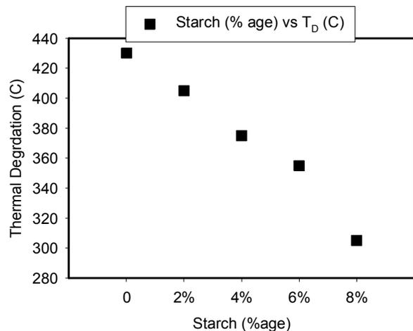
Fig. 5. Relationship of thermal degradation temperature and starch content.
