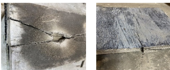
Fig. 5. Typical failure behavior of reinforced concrete slabs.
