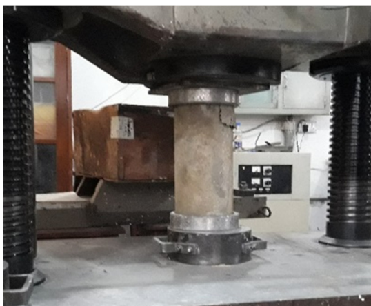
Fig. 1. Concrete cylinder test setup.
