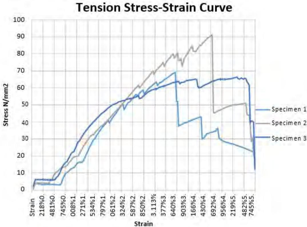
Figure 21. Tensile Stress-Strain Curves of the 3 specimens
