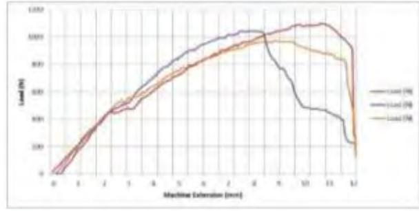
Figure 38. Graphs of the apparent Modulus of Elasticity of span 280 mm (Author's own, n.d.)
