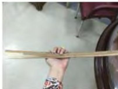
Figure 25. The longitudinal cracking in a specimen (Author's own, n.d.)
