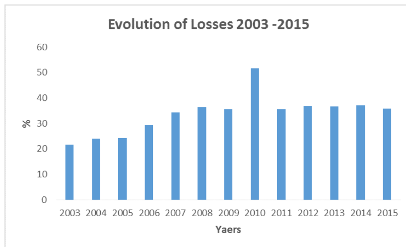
Figure 5. Evolution of Santiago Island electrical losses.
