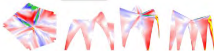
Figure 6. Karamba structural analysis showing areas of compression (Red), tension (Blue), maximum tension (green), maximum compression (yellow), and neutral areas (white).
