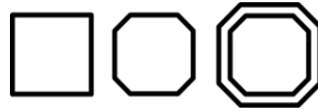
Fig. 2 Used trench tub layout geometries in top down view: 90° trench corner angle (left), 135° trench corner angle (center) and 135° double trench corner angle (right)
