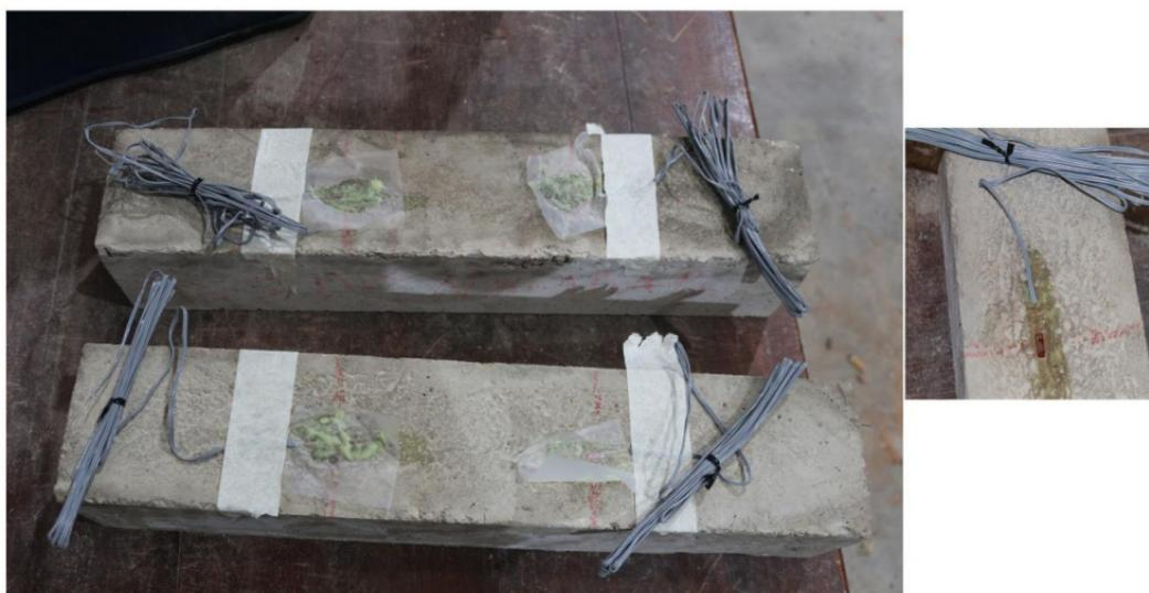
Figure 7: Strain gauges installed on concrete beam.
