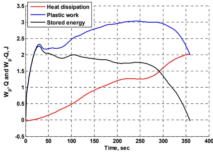
Figure 5: Time dependence of plastic work, heat dissipation energy and stored energy.
