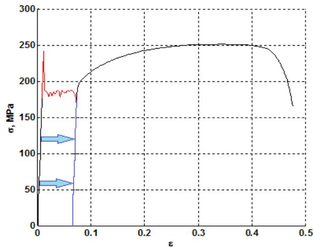
Figure 7: Experimental stress-strain curve for Armco iron.
