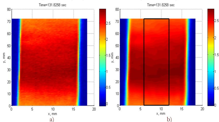
Figure 3: Temperature range on the surface of specimen before data processing (a) and obtained field of temperature range with zone of interest (b).
