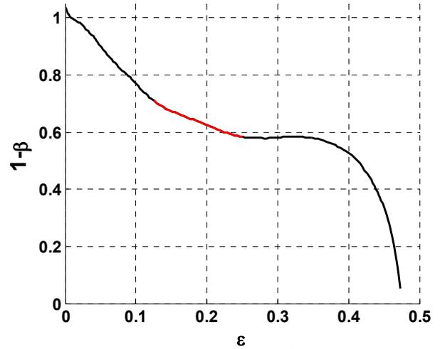
Figure 6: Strain dependences of stored energy ratio  $(1-\beta)$ .
