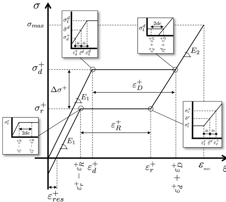
Figure 3: Stress  $\sigma$  vs. strain  $\varepsilon$  predicted by present model in a displacement-driven traction loading-unloading test at the high temperature  $T_2 > T_{af}$ . The applied strain is depicted in Fig. 2 for  $\tau \in [0, 2t_1]$ .
