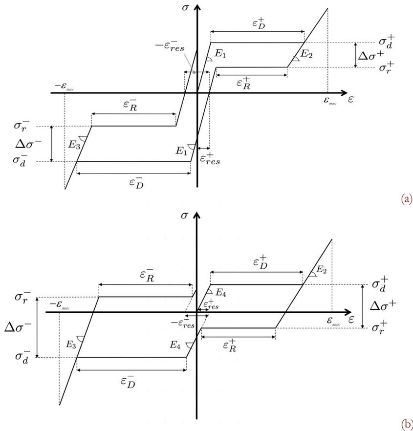
Figure 5: Stress  $\sigma$  vs. strain  $\varepsilon$  predicted by present model in a tensile-compressive loading-unloading test obtained from applied strain as in Fig. 2 at the high temperature  $T_2$  (a) and at the low temperature  $T_1$  (b).
