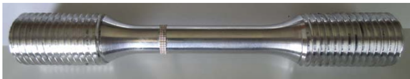
Figure 1: Specimen used for fatigue crack growth data.
