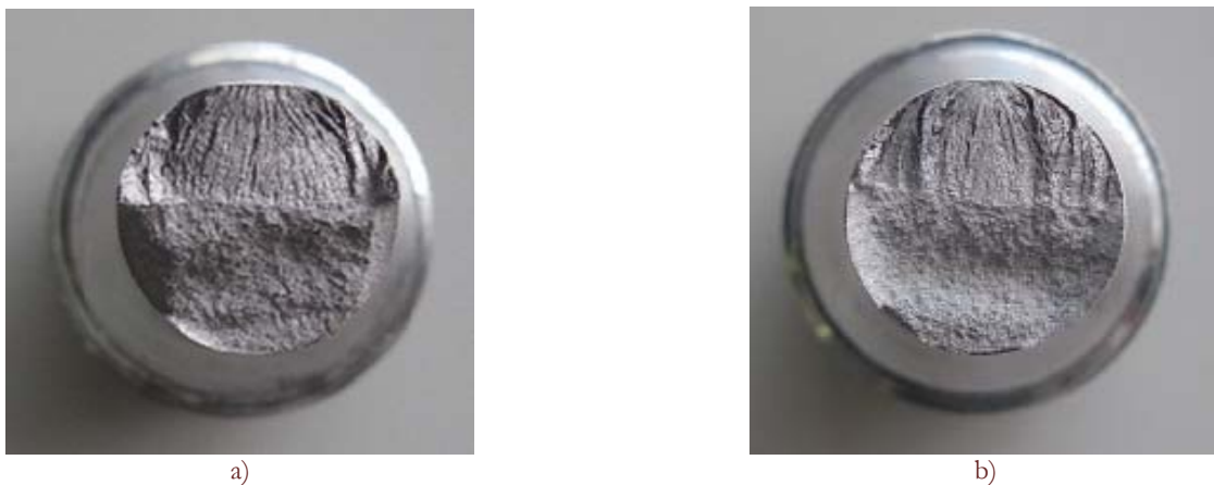
Figure 3: Fracture surfaces for: a) pure rotating bending (symmetrical crack growth); b) rotating bending with steady torsion (nonsymmetrical crack growth).
