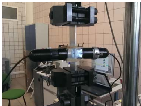
Figure 5: Microscopes attached to the specimen surface.
