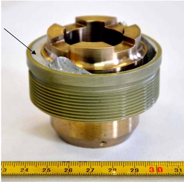
Figure 2: Cap entangled inside the fracture surface.
