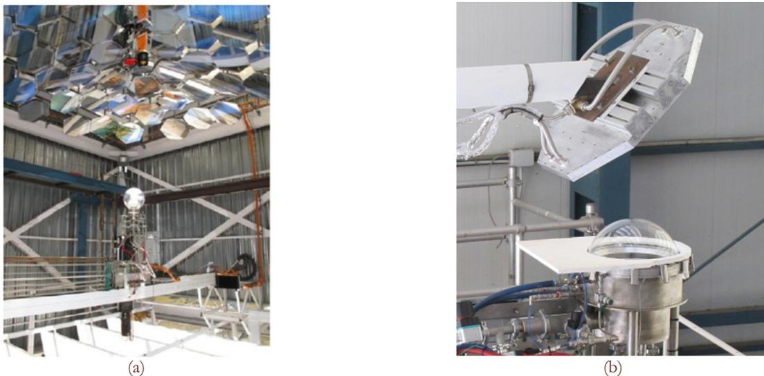
Figure 2: Examples of glass components of CSP systems at PSA-CIEMAT. a) Aspect of the solar concentrator and reaction chamber of SF-5 solar furnace; b) Aspect of the MiniVac chamber installed at the focal spot of the new SF-40 solar furnace; a 45° inclined mirror above the MiniVac allows the sunrays to reflect vertically.
