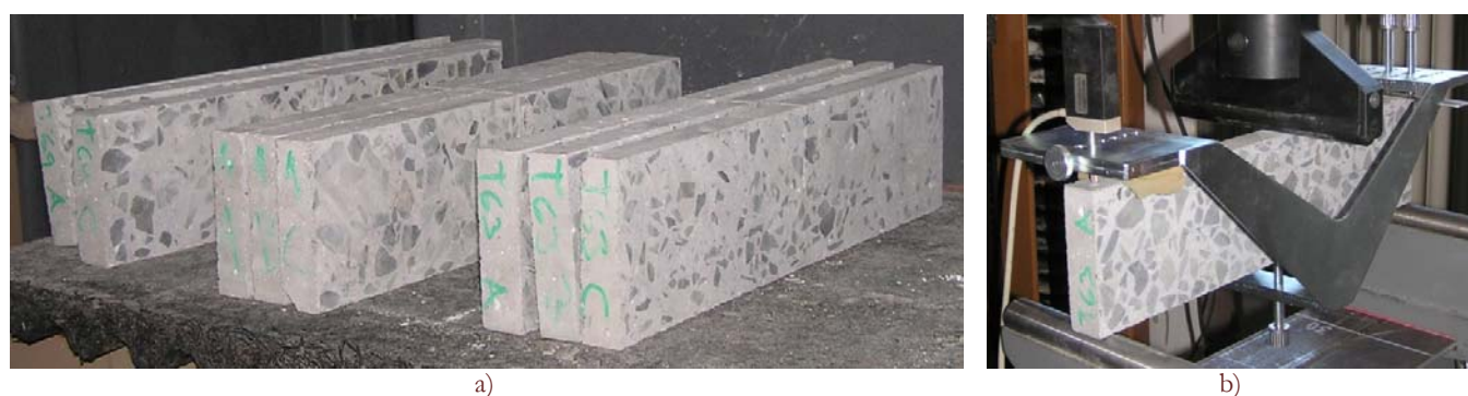
Figure 1: a) Preparation of notched specimens for bending test from standard beams, b) employed fracture test geometry – three-point bending of notched beam – with a depiction of the measuring fixture enabling recording of pure beam deflection.
