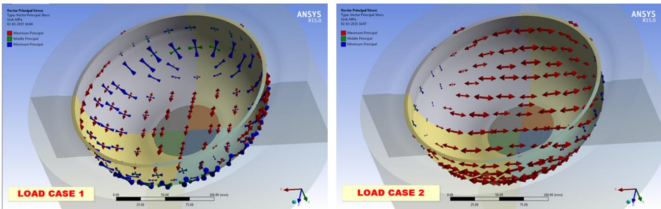
Figure 3: Stress distribution at minimum et maximum of fatigue loading.
