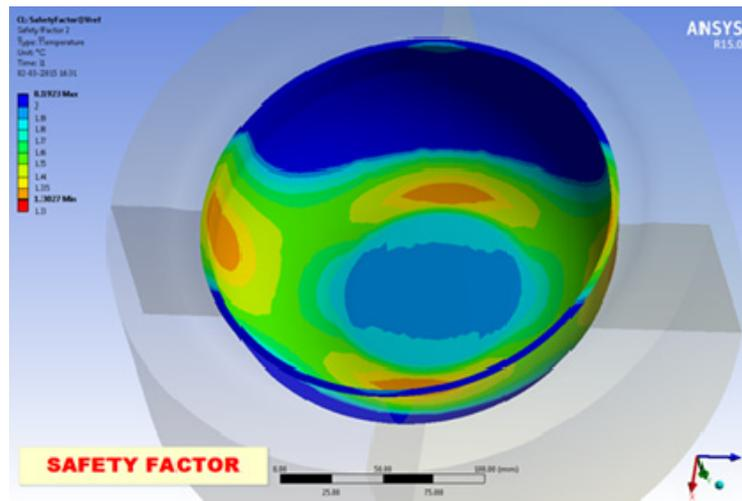
Figure 4: Safety factor and final result of the overall investigation.
