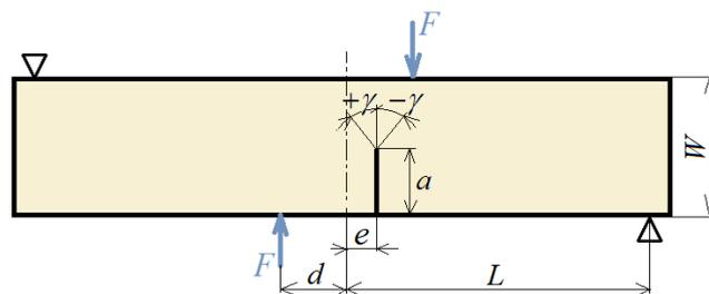
Figure 1: Eccentric asymmetric four point bending of a notched beam specimen under study.
