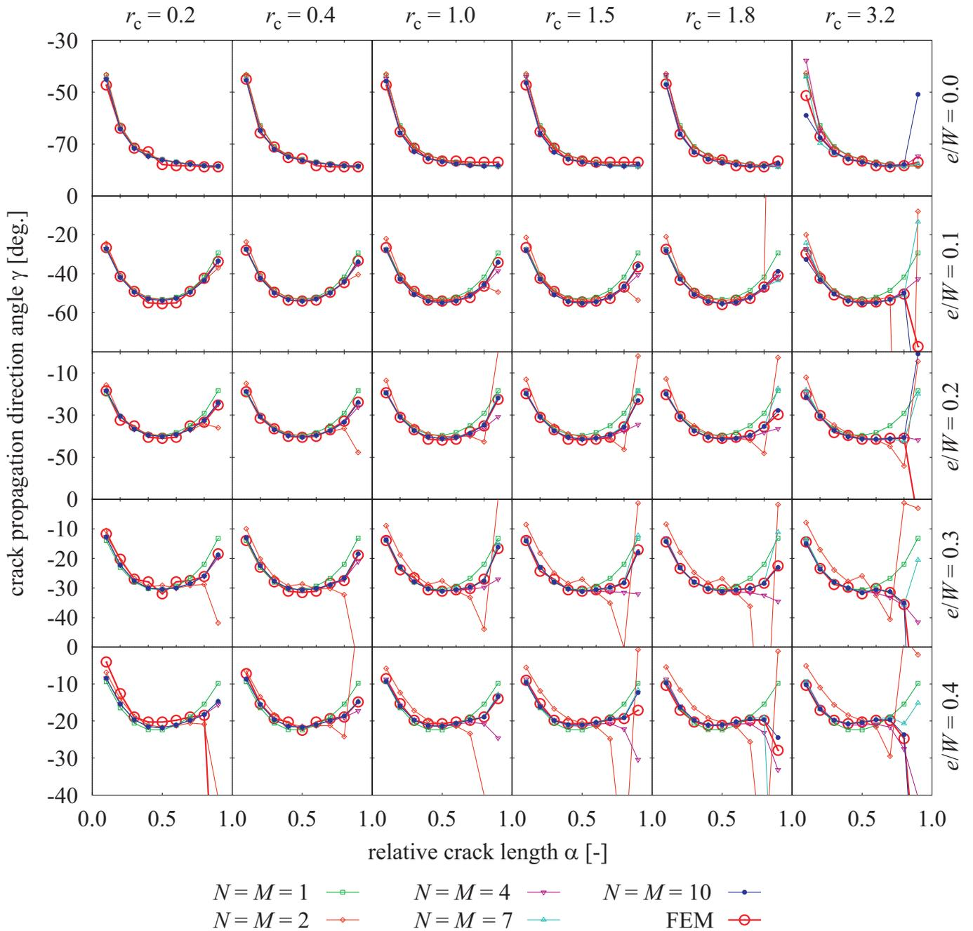
Figure 3: Dependences of the initial crack propagation direction angle  $\gamma$  on the relative crack length  $\alpha$  for various relative crack eccentricities  $e/W$  obtained from the SED fracture criterion at various radial distances from the crack tip  $r_c$ ; the purely numerical results ("FEM") are compared to the semi-analytical results (" $N = M = 1, 2, 4, 7$  and  $10$ ") calculated via the multi-parameter form of the fracture criterion.
