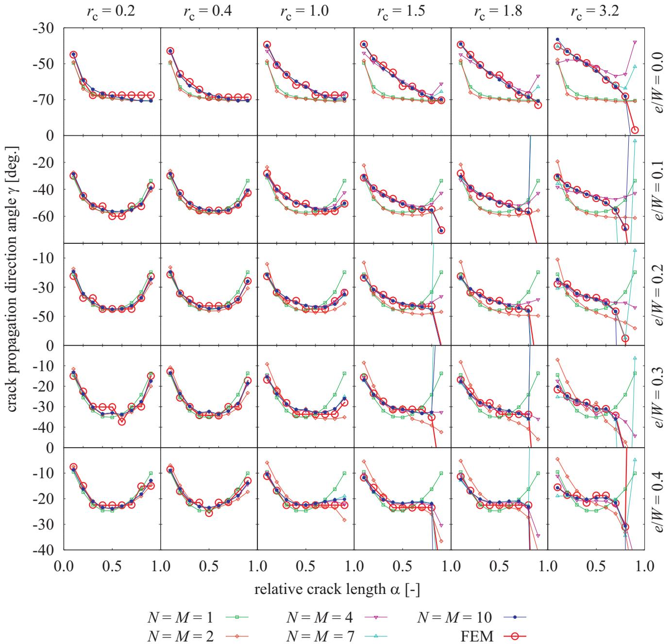
Figure 2: Dependences of the initial crack propagation direction angle  $\gamma$  on the relative crack length  $\alpha$  for various relative crack eccentricities  $e/W$  obtained from the MTS fracture criterion at various radial distances from the crack tip  $r_c$ ; the purely numerical results ("FEM") are compared to the semi-analytical results ("N = M = 1, 2, 4, 7 and 10") calculated via the multi-parameter form of the fracture criterion.
