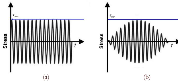
Figure 9: Two different loading paths with same maximum stress.
