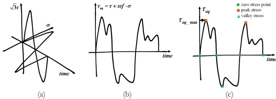
Figure 10: Virtual cycle counting variables identification.
