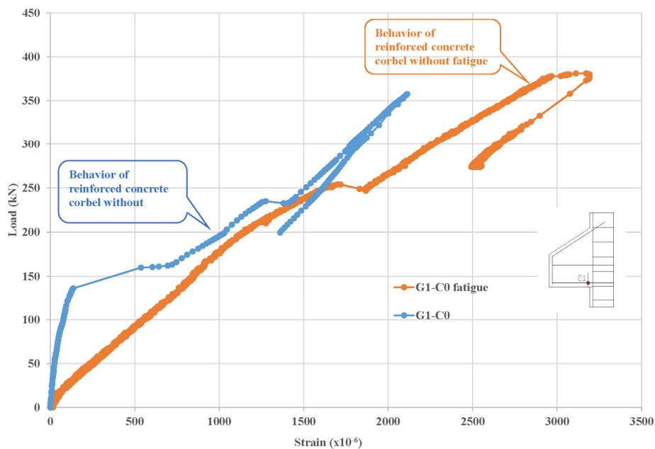
Figure 4: Effect of fatigue on reinforced concrete corbels under static tests.
