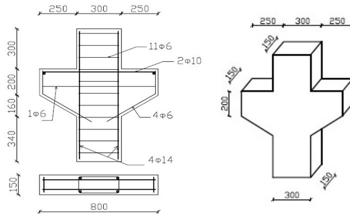
Figure 1: Details of corbel geometry and steel frame.
