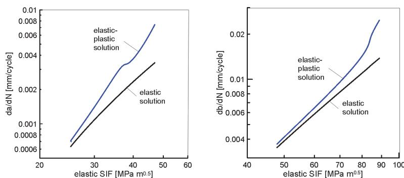
Figure 7: Crack growth rate comparison for elastic and elastic-plastic solutions.
