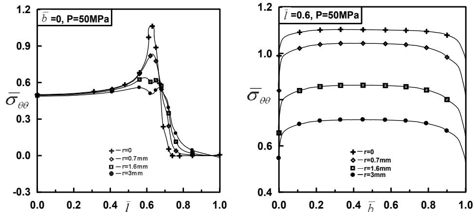
Figure 4: Hoop stress distributions along fillet and hub.
