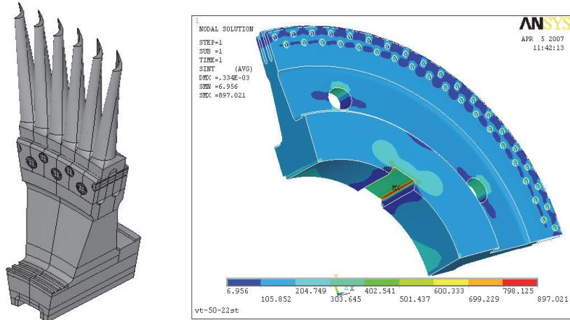
Figure 2: Equivalent stress distribution for turbine disk.
