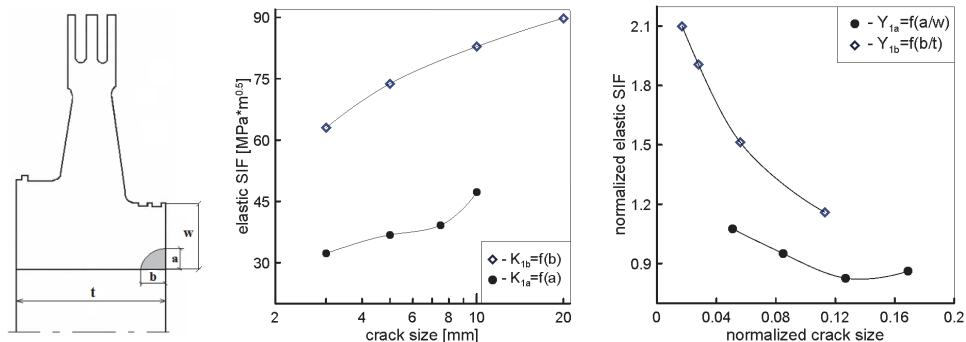
Figure 5: Elastic SIF versus crack size in depth and length direction.
