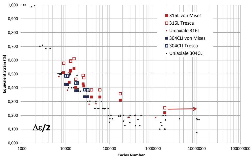
Figure 5: Austenitic stainless steel fatigue curve for 304L-CLI and 316L under uniaxial and equibiaxial loadings
