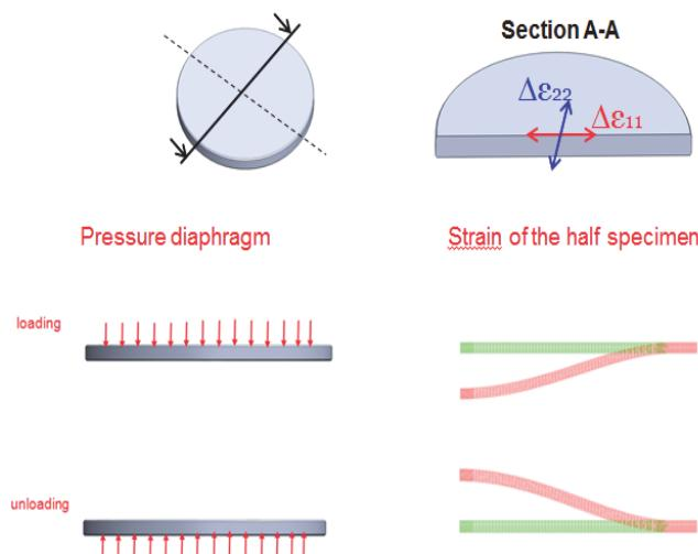
Figure 1: Principle of the new experimental fatigue test.
