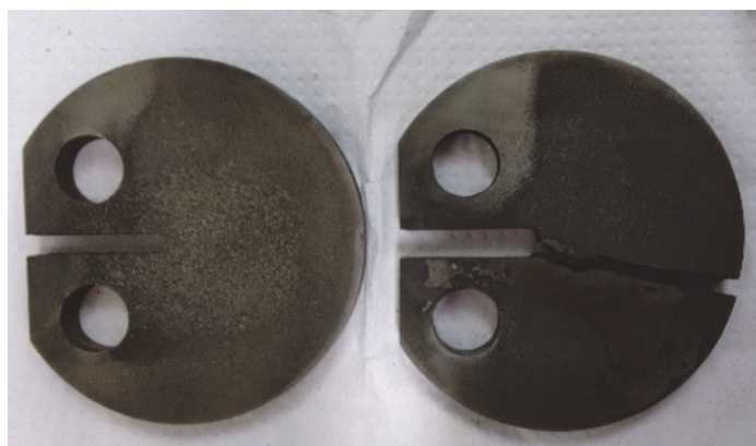
Figure 7: LE specimens after working 30 days under EAC conditions in an aqueous hydrogen sulfide environment.
