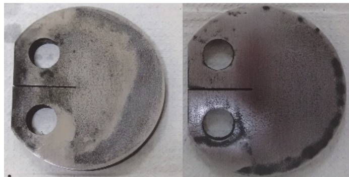
Figure 10: EP specimens after 30 days under EAC in aqueous hydrogen sulfide environment.
