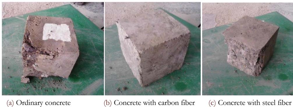
Figure 11: Damage situation of the two different test blocks after the pressure test
