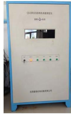
(b) Thermal conductivity tester
