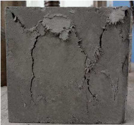
Figure 1: Failure mode of test specimens.
