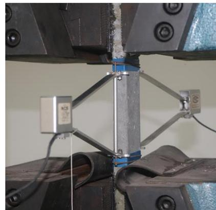
Figure 4: Experimental set-up for uniaxial tensile test.
