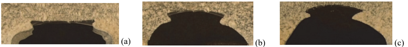
Figure 4: Crack tip splitting at the incipient failure for specimens (a) C2b, (b) C3b and (c) C4b.
