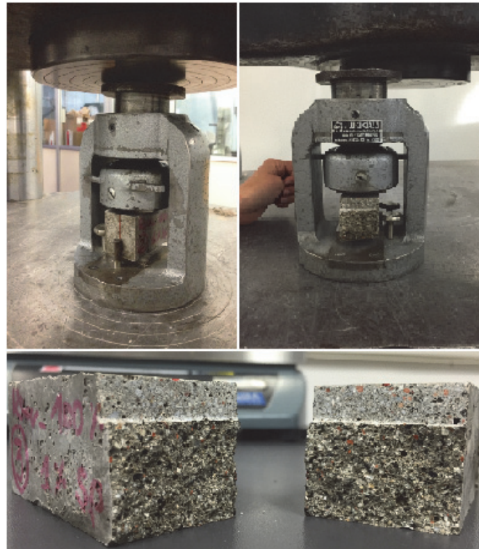
Figure 5: Set up and test of experimental mortars: compression test.
