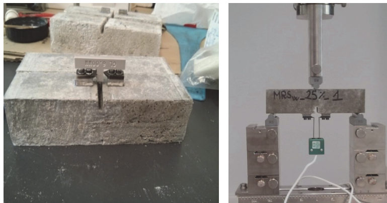
Figure 4: Set up and test of experimental mortars: three-point bending test.
