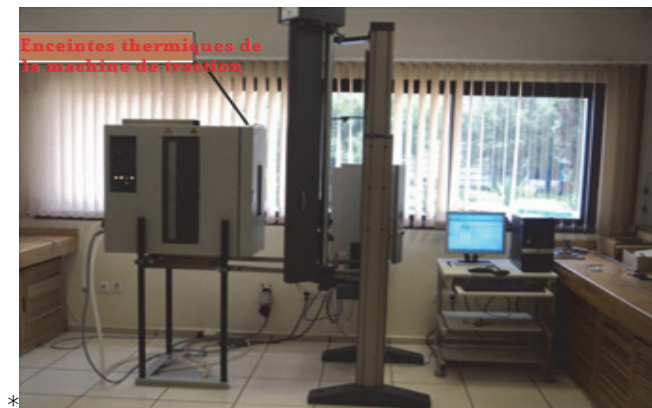
Figure 3: Thermal enclosure assembly with tensile test machine.
