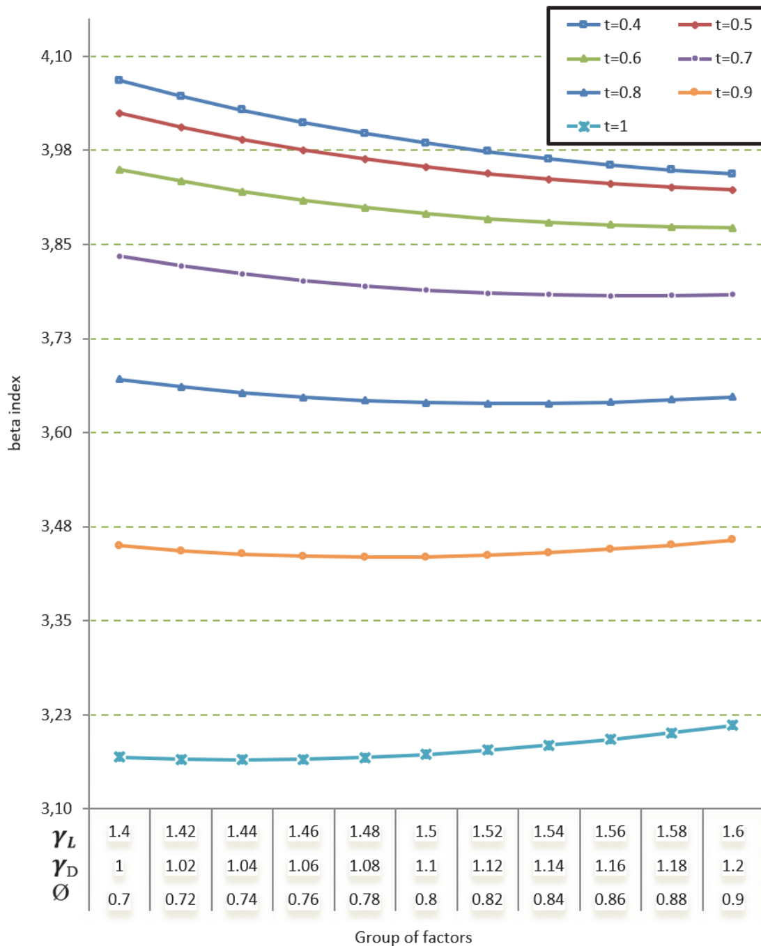
Figure 9: Prediction of load and resistance factors for the L section beam in combined state
