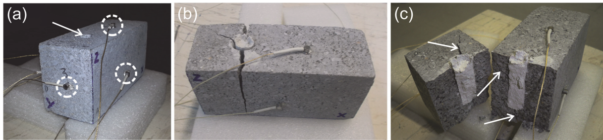
Figure 1: (a) The concrete specimen with the AE sensors mounted on it. The arrow indicates the pre-drilled hole filled with the expansive mortar and the dashed circles indicate the positions of the visible AE sensors; (b) The concrete block at the end of the monitoring where the fracture plane is parallel to the y-z plane; (c) View of the two splitting pieces of the concrete block after its ultimate rupture. White arrows indicate main visible macro-cracks.
