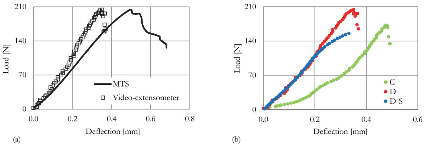
Figure 7: (a) The load-deflection curves obtained by the video-extensometer and the loading frame for a typical diabetic femur; (b) typical load-deflection curves for the three animal groups of the present study.
