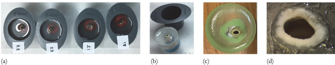
Figure 3: (a) The fractured bones surrounded by the resin in the plastic caps; (b,c) Typical bone-resin construct; (d) Photo of the polished surface of a typical construct.
