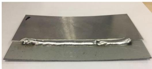
(a) Post-weld plate without reverse deformation treatment
