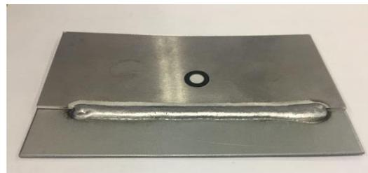
(c) Post-weld plate for GA-BPNN reverse deformation treatment
