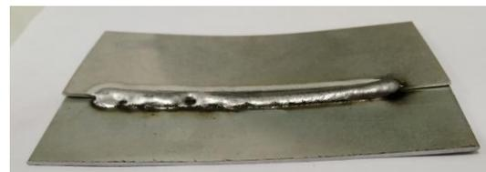
(b) Post-weld plate of BPNN reverse deformation treatment
