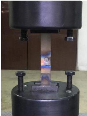
Figure 9: Clamping specimen.
