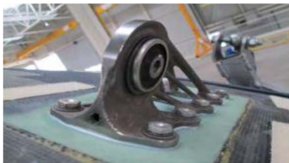
Figure 2: Airbus ALM/3D printing FCRC cabin bracket installation [14][15].
