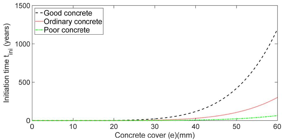
Figure 10: Effect of concrete cover, and quality of concrete on initiation time of corrosion.
