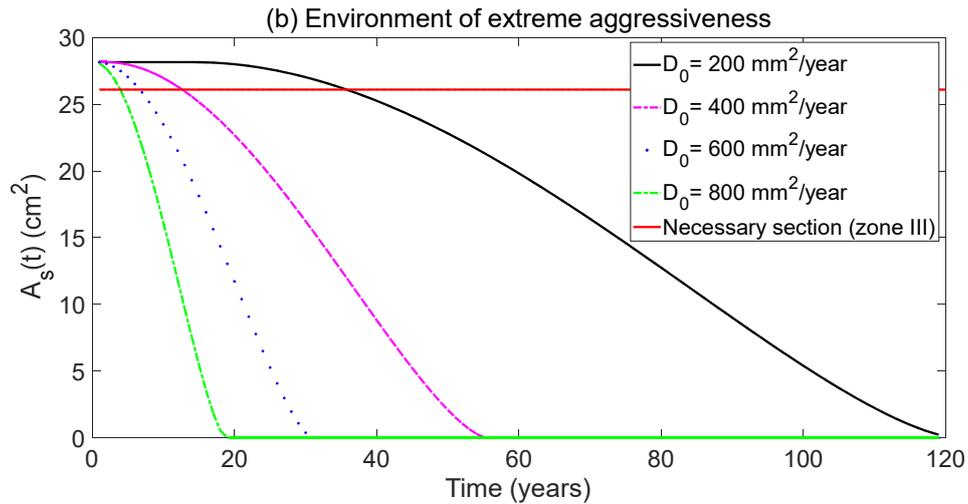
Figure 9: Evolution of residual section of reinforcements for different diffusion coefficients.
