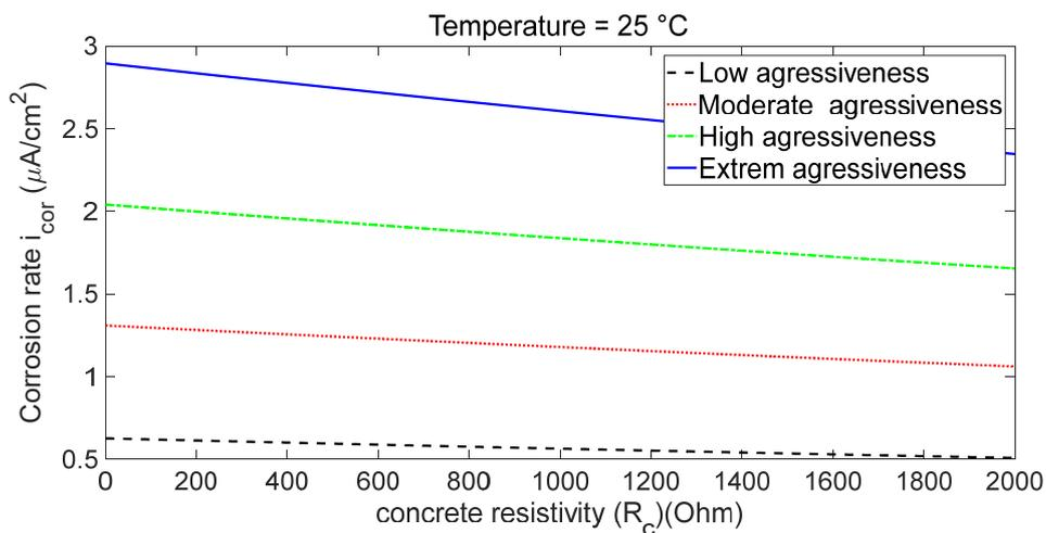
Figure 16: Effect of the concrete resistivity and the concentration of chlorides ions on the corrosion rate.
