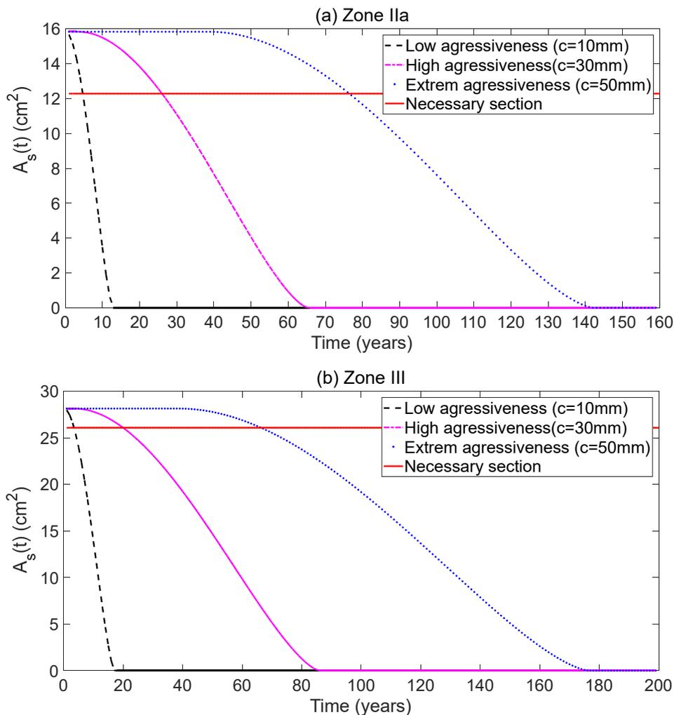
Figure 7: Evolution of the reinforcements section for different concrete covers recommended by BAEL [29].
