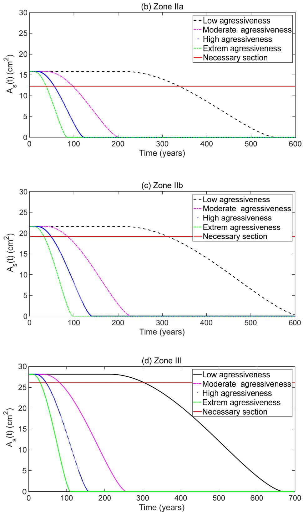
Figure 5: Evolution of the reinforcements section as a function of time for different seismic zones.
