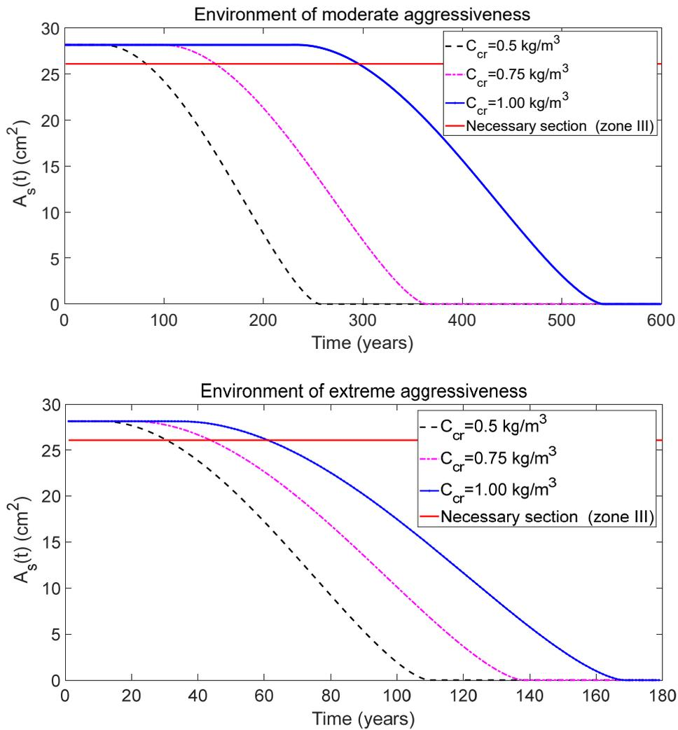
Figure 13: Evolution of the residual section of reinforcements for different values of the critical concentration.
