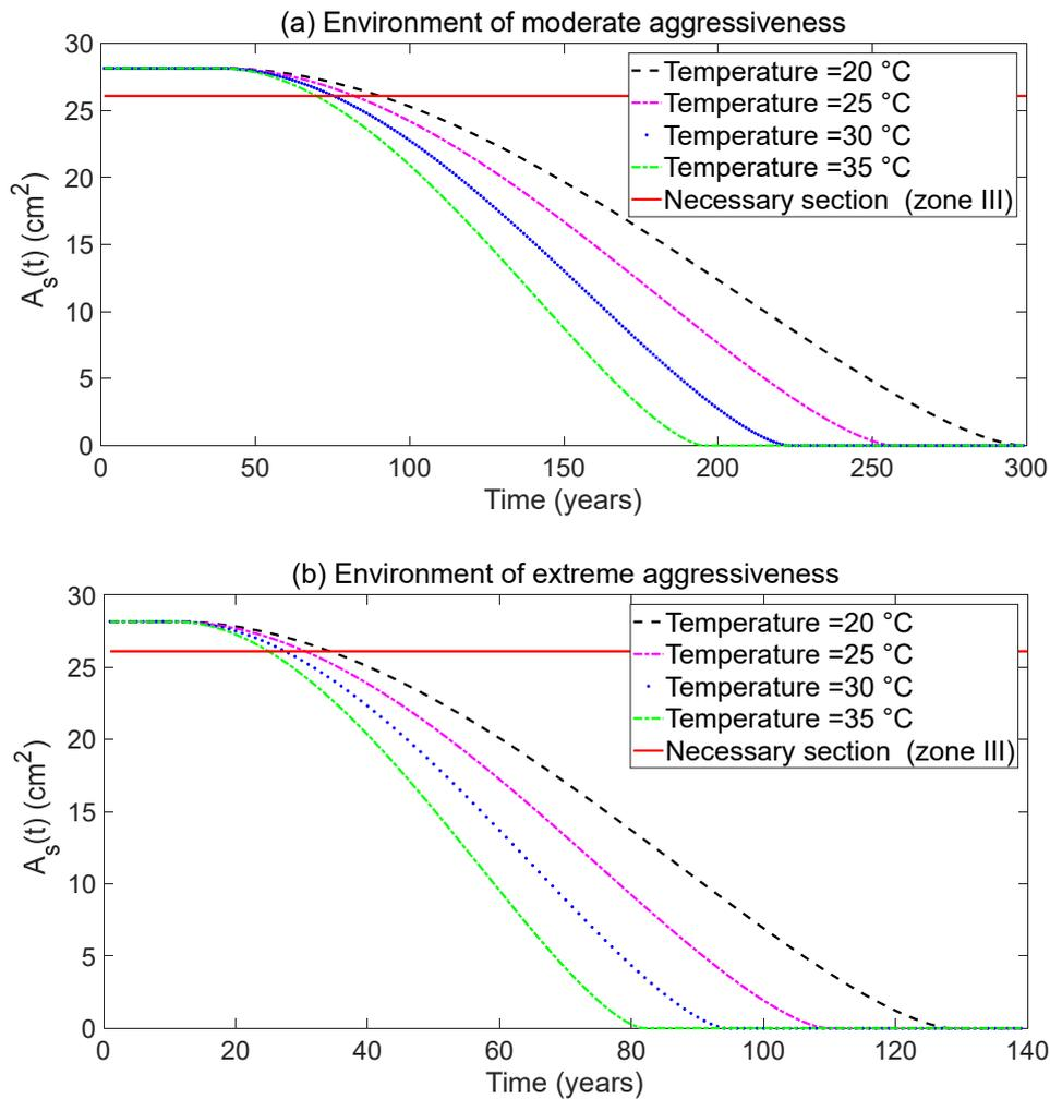
Figure 15: Evolution of the residual section of reinforcements for different temperature values.
