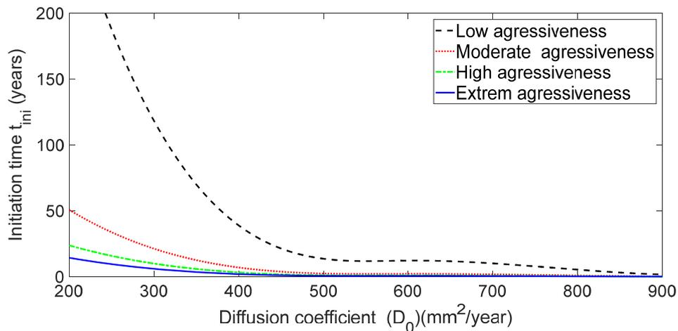
Figure 8: Effect of diffusion coefficient and chloride ion concentration on corrosion initiation time.
