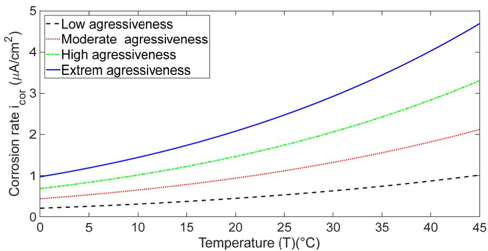
Figure 14: Effect of Temperature on corrosion rate for different concentrations of chlorides ions.
