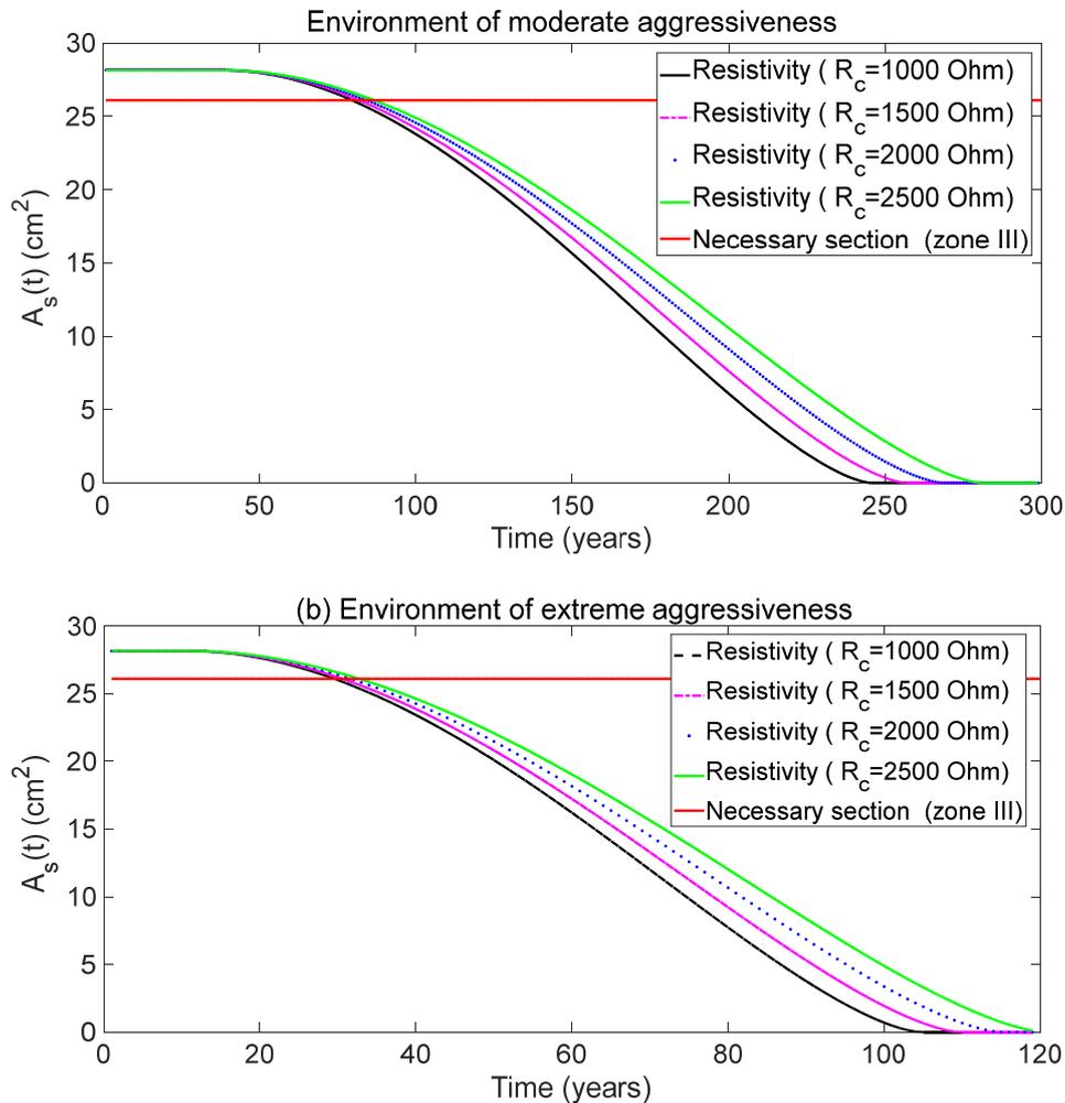
Figure 17: Evolution of the residual section of reinforcements for different resistivity values.
