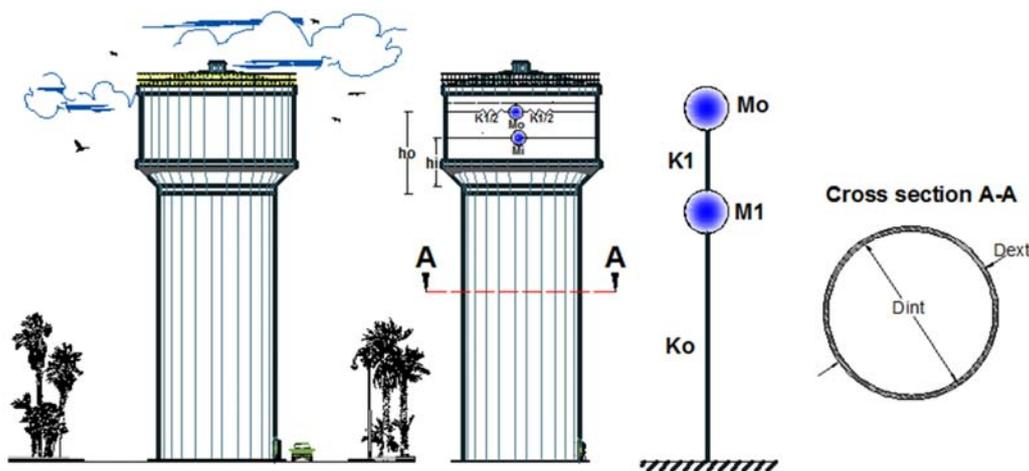
Figure 2: Elevated tank - equivalent mechanical and mathematical models.
