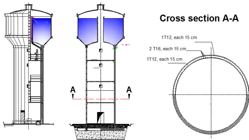
Figure 4: The studied elevated tank with the adopted reinforcement of the pedestal in a very high seismicity zone.
