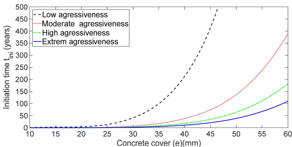
Figure 6: Evolution of initiation time as a function of concrete cover, for different environments.
