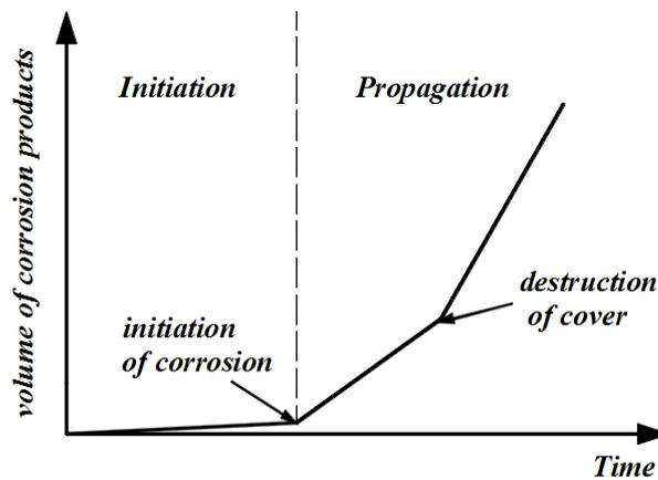
Figure 1: Schematic degradation of steel reinforcement over time [17].
