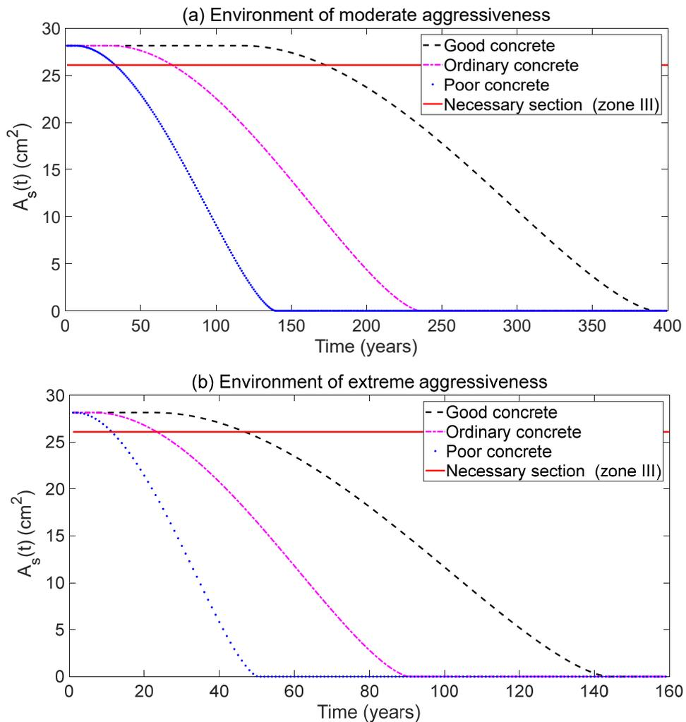
Figure 11: Evolution of residual section of reinforcements as a function of time for different cement contents.
