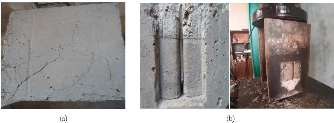
Figure 6: Failure modes. (a) Concrete crushing, (b) Shearing of the connector.
