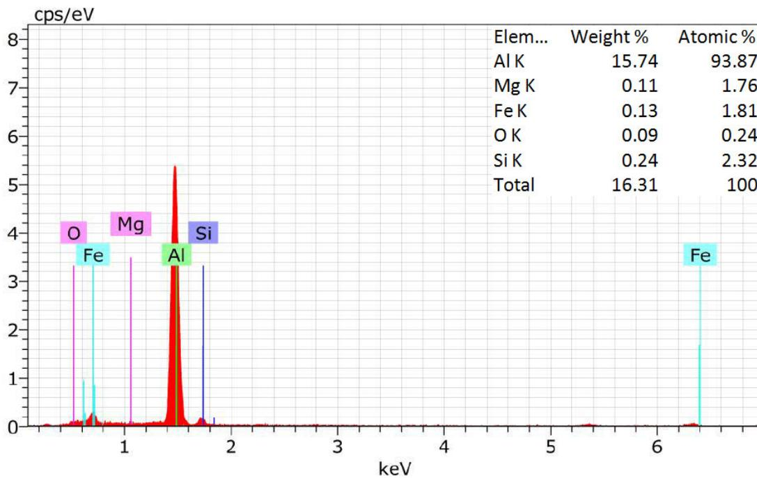
Figure 2(a): EDX spectrum of the Al6061-8wt%Flyash
