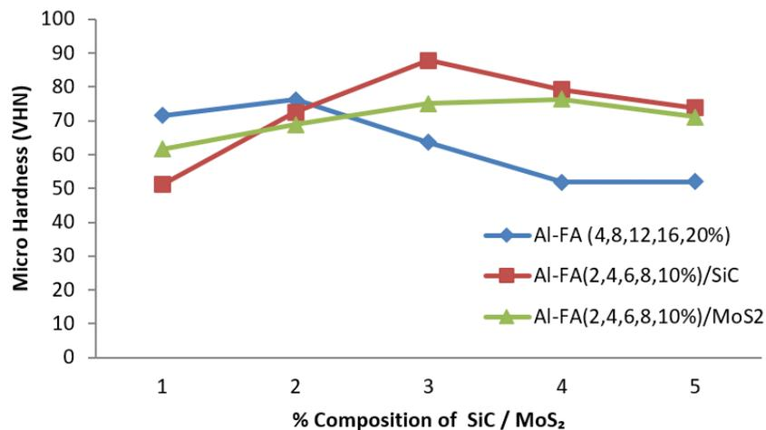
Figure 5: Micro-hardness of hybrid aluminum matrix composites
