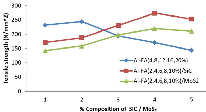
Figure 6: Tensile strength of hybrid aluminum matrix composites.
