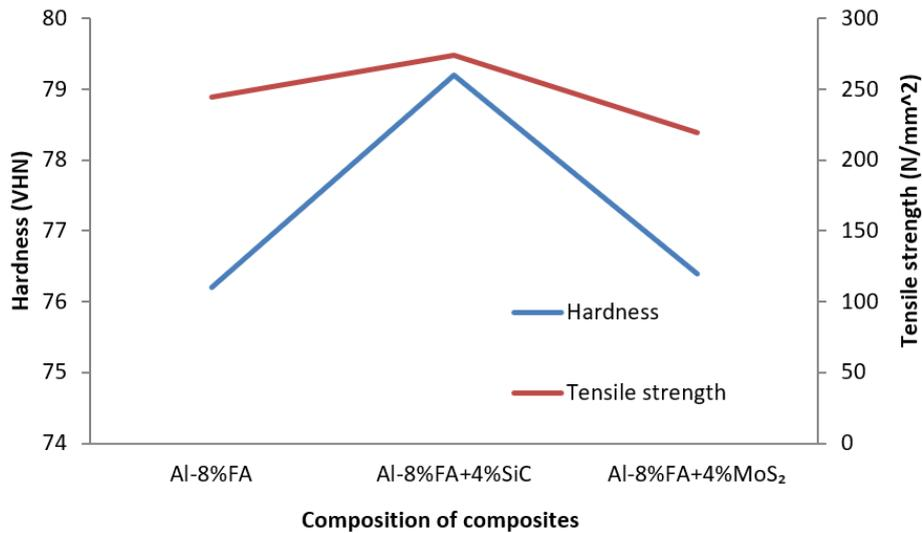
Figure 7: Comparison of hardness and tensile strength of composites at 8wt% of the flyash
