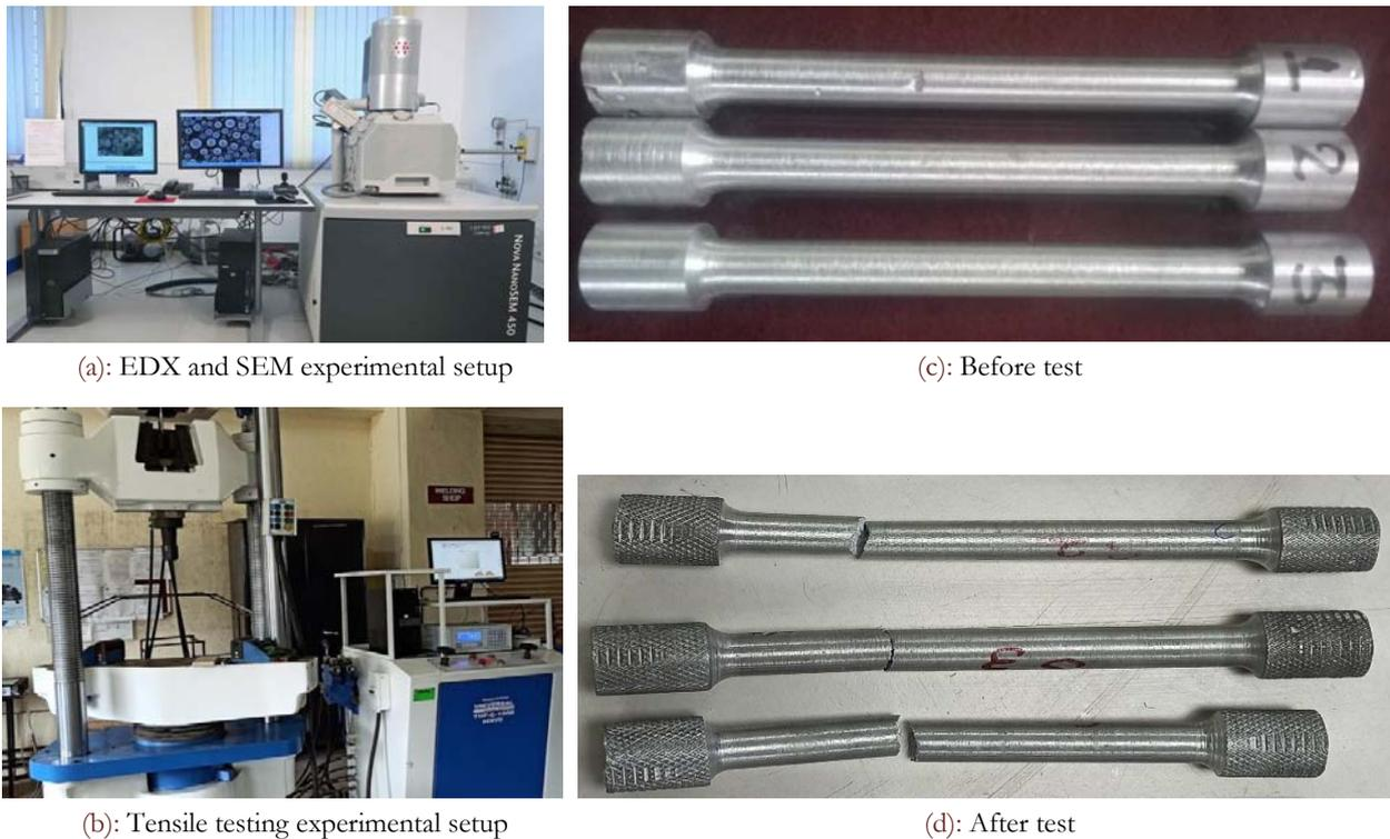
Figure 1 (a): EDX and SEM setup, (b) Tensile testing setup, (c-d): Tensile test specimens Al6061-Flyash composites.
