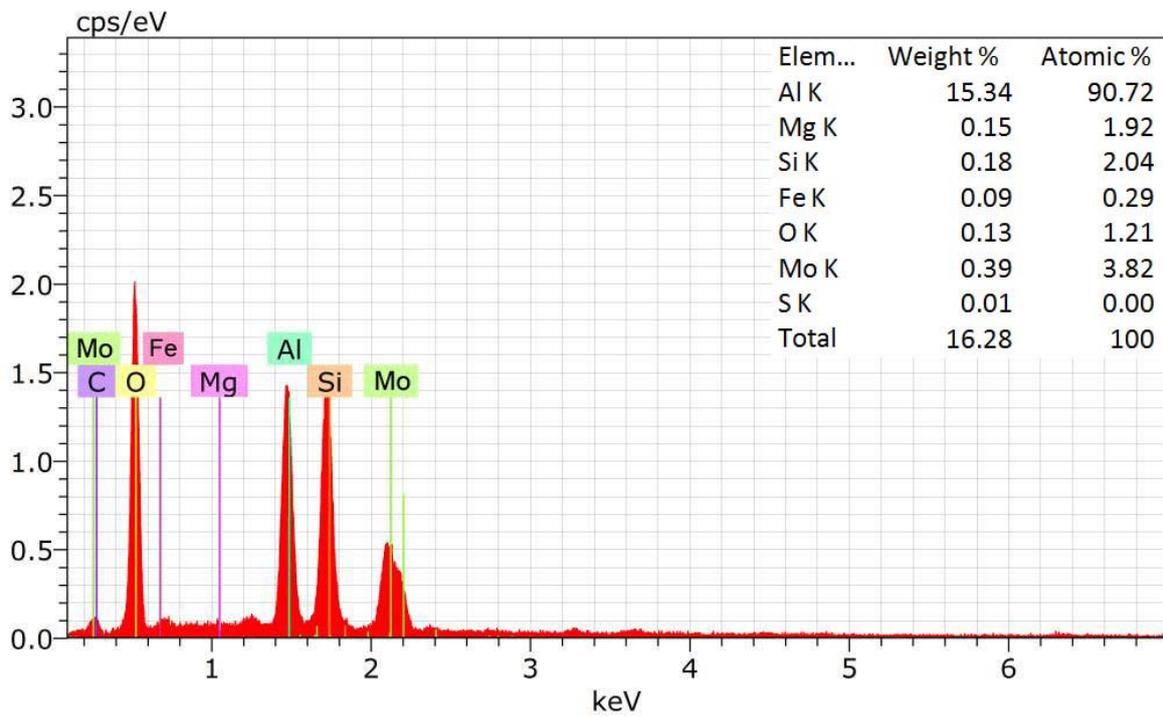
Figure 2(c): EDX spectrum of the Al6061-6wt%FA/ 3wt%MoS<sub>2</sub> composite.
