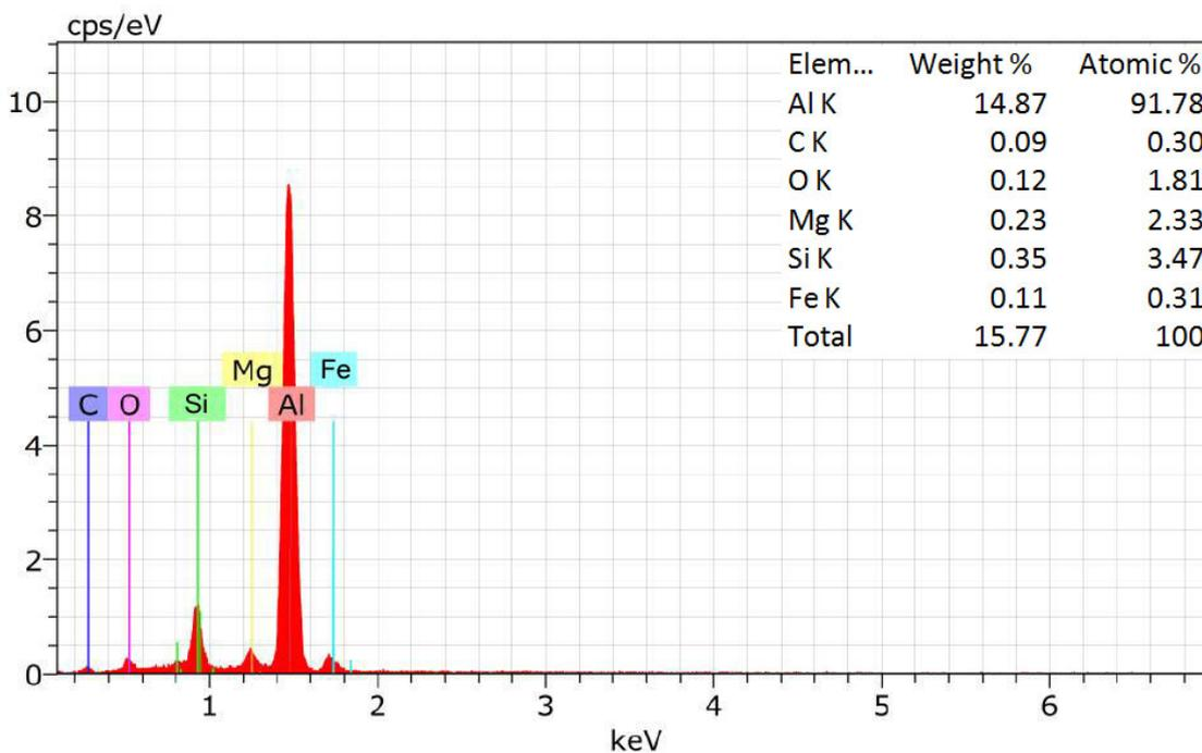
Figure 2(b): EDX spectrum of the Al6061-6wt%FA/ 3wt%SiC composite.
