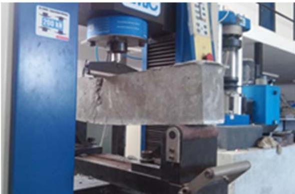
Figure 3: Beam during the test.
