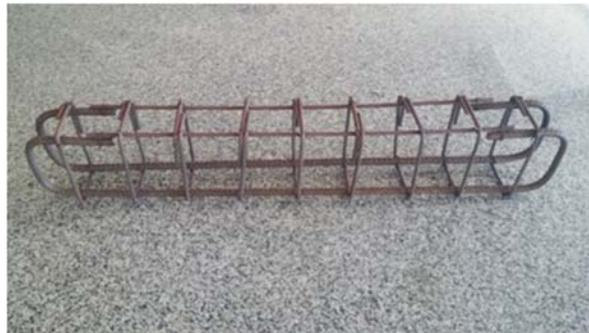
Figure 1: Reinforcement of the beam.
