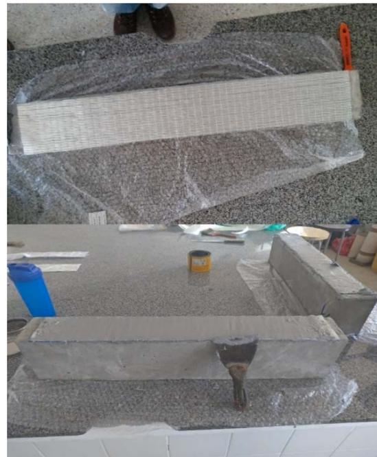
Figure 4: Glass fibre application.
