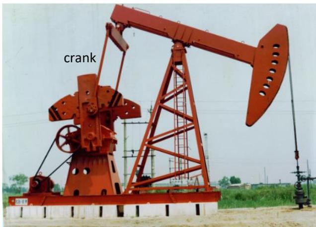
Figure 1: The conventional beam pumping unit
