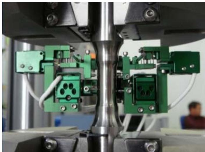
Figure 2: The biaxial servo-hydraulic test system Instron 8850 (left), the biaxial extensometer Epsilon 3550-025M (right).
