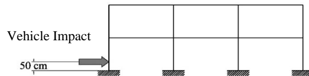
Figure 4: Location of vehicle impact to corner column.
