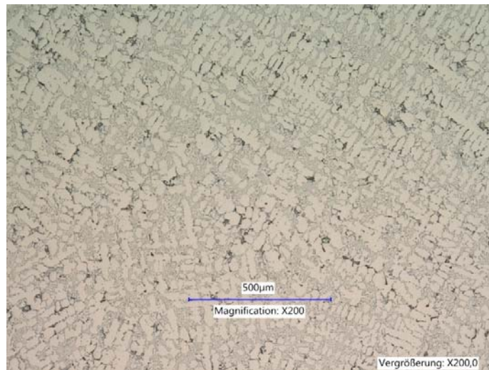
Figure 2: Optical micrograph images of AlSi samples with 200X magnification.
